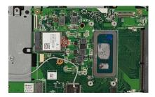
**13.** Remove 7 screws that secures the motherboard to top case then lift the motherboard off the alignment pins and remove it from top case.
