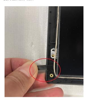
27. Lift the panel off the LCD back cover and set it in front of the LCD back cover
