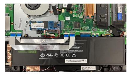
**3.** Disconnect the fan cable from the connector on the motherboard. Remove the 7 screws that secures the heatsink and fan module to the motherboard and top case. Then lift the thermal module off the standoffs on the motherboard.
