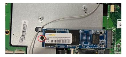
**10.** Peel off the acetate tape that secures the memory module then push both arms outward simultaneously to release the memory module to the spring tension position. Grasp the memory module by the edges and pull gently to remove it from the slot on the motherboard.
