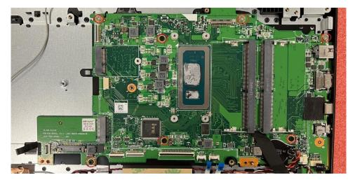
**14.** Remove 1 screw that secures the LTE module to the I/O board then remove it from I/O board.
