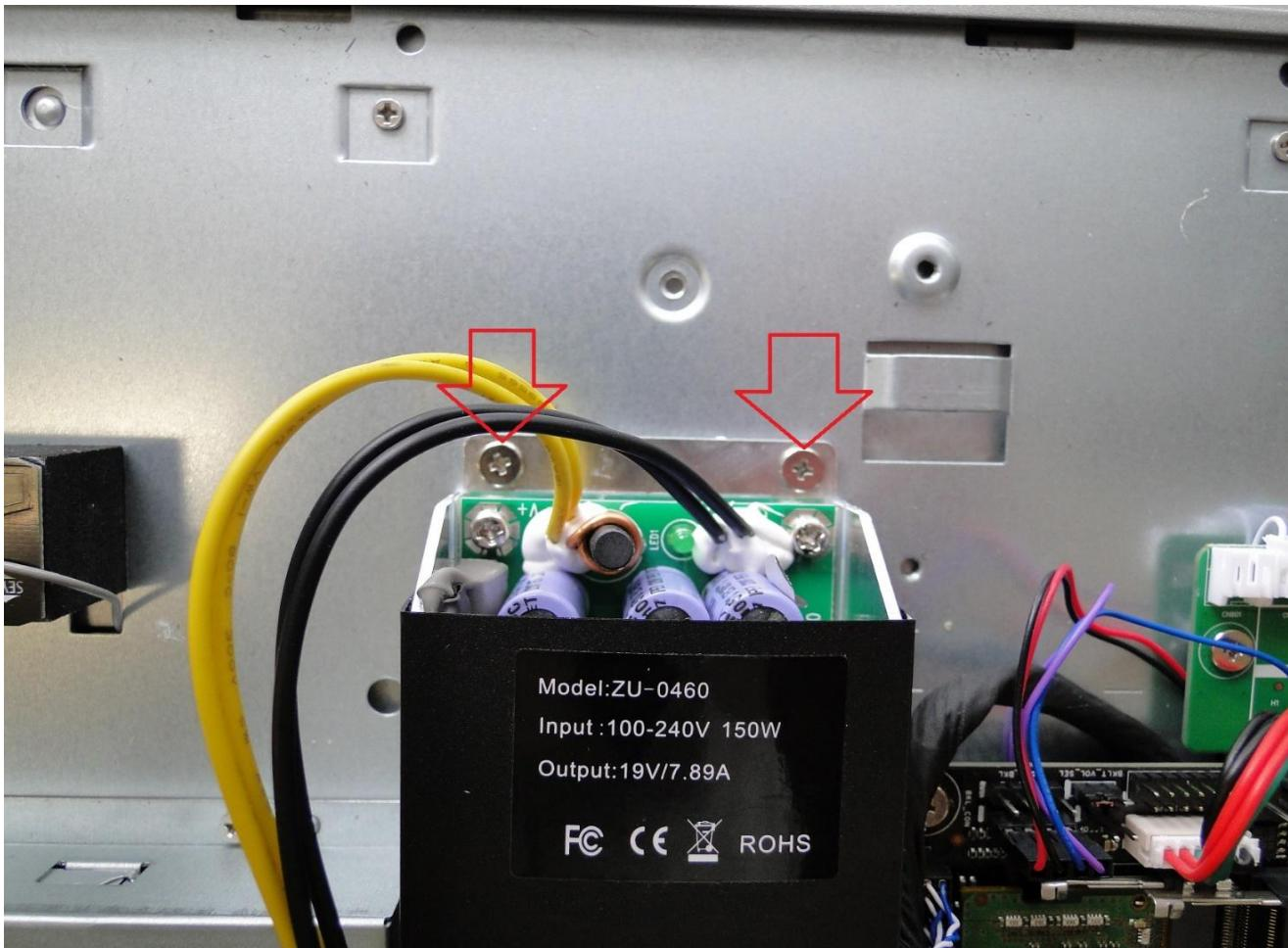
Using a Philips screwdriver, detach the 2 screws securing the power supply socket.
