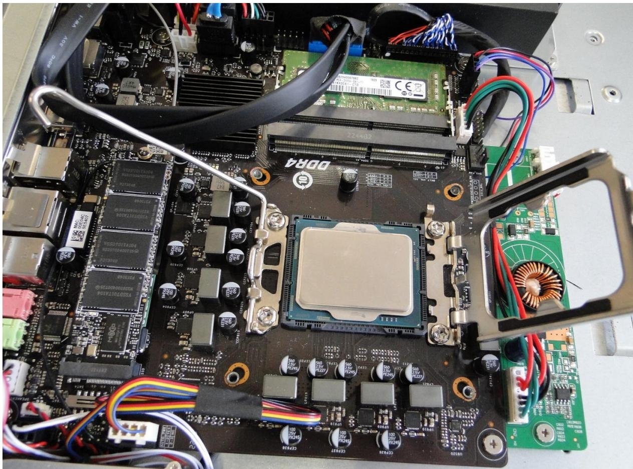
Carefully lift the CPU with your fingers and remove it from the base
