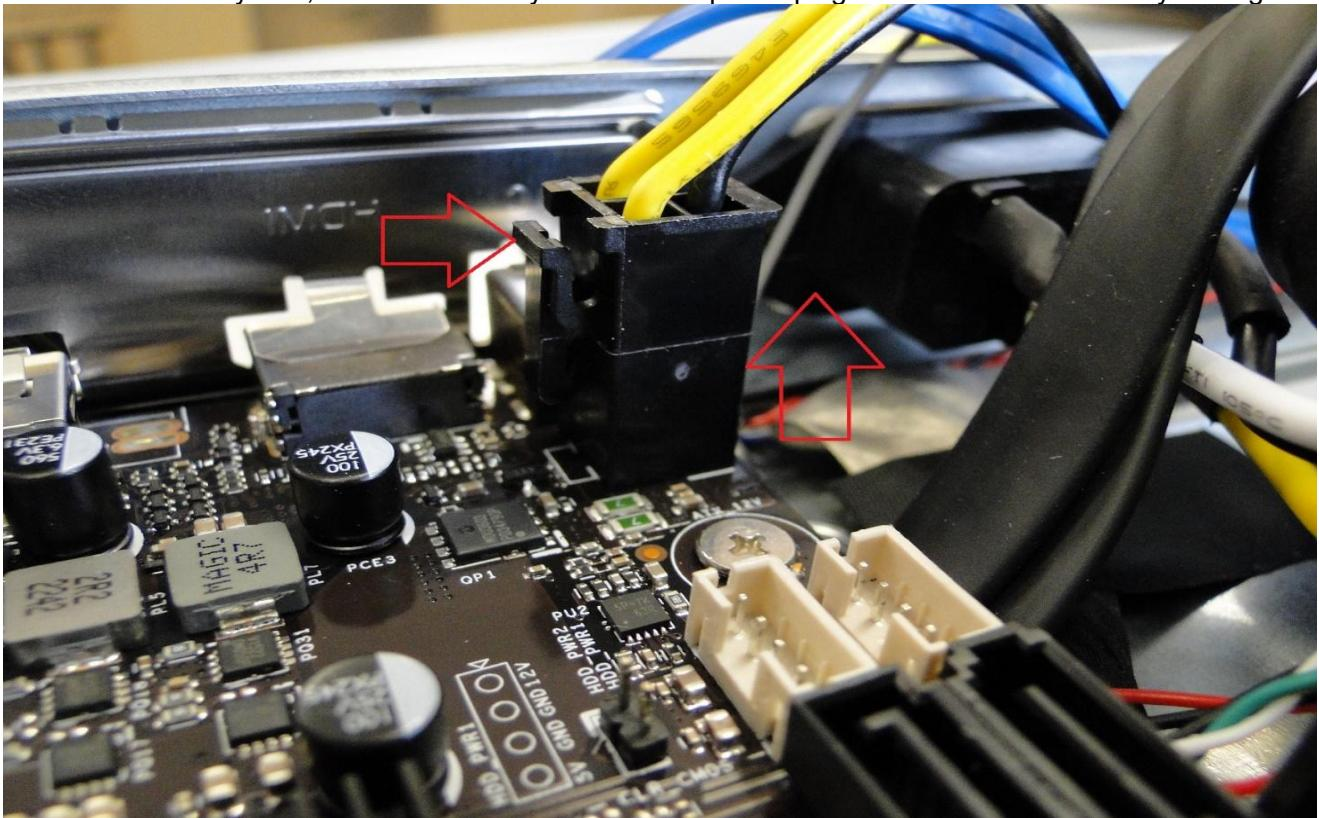
Carry out the assembly in a reverse order. When connecting the power plug of the motherboard, pay attention to the alignment of the symmetrical points.
