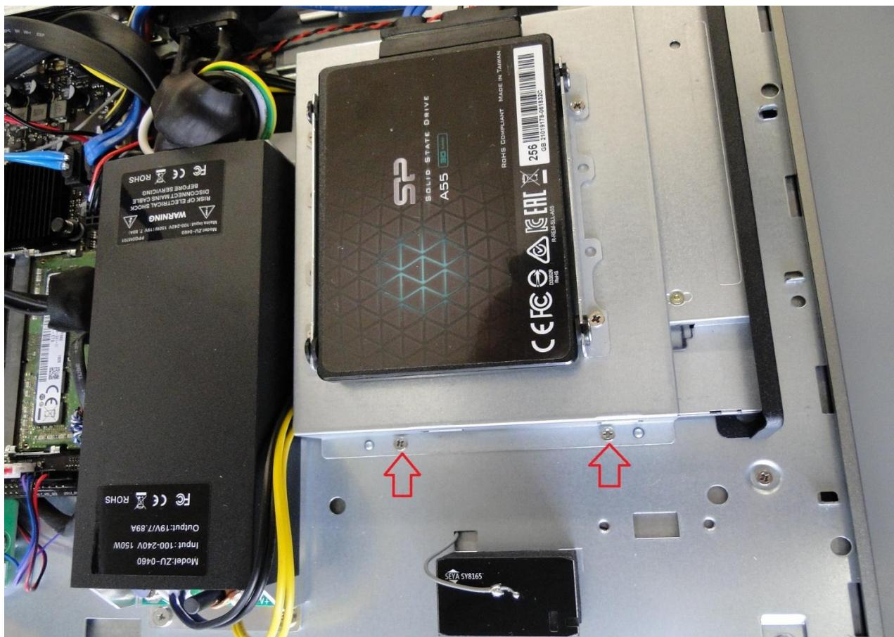
Lift the back of the optical drive case upward.
