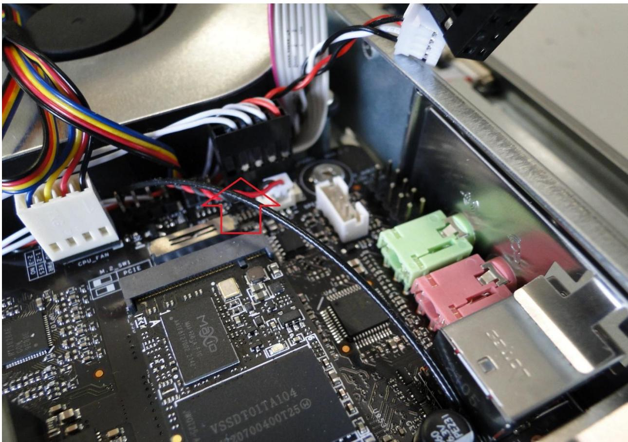
**Removal of the processor cooling system harness**
