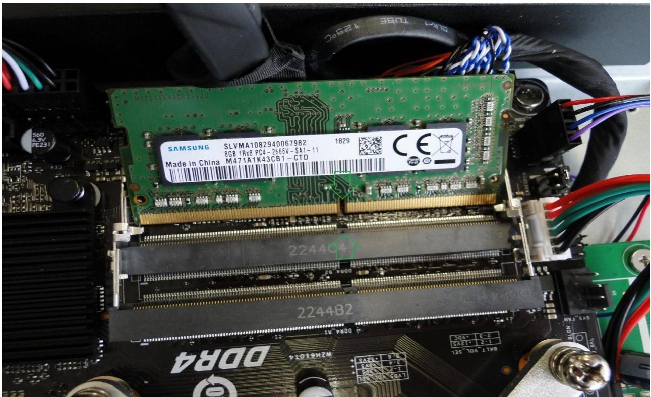
Correct assembly involves inserting the memory module into the socket and pressing down to snap it into place.
