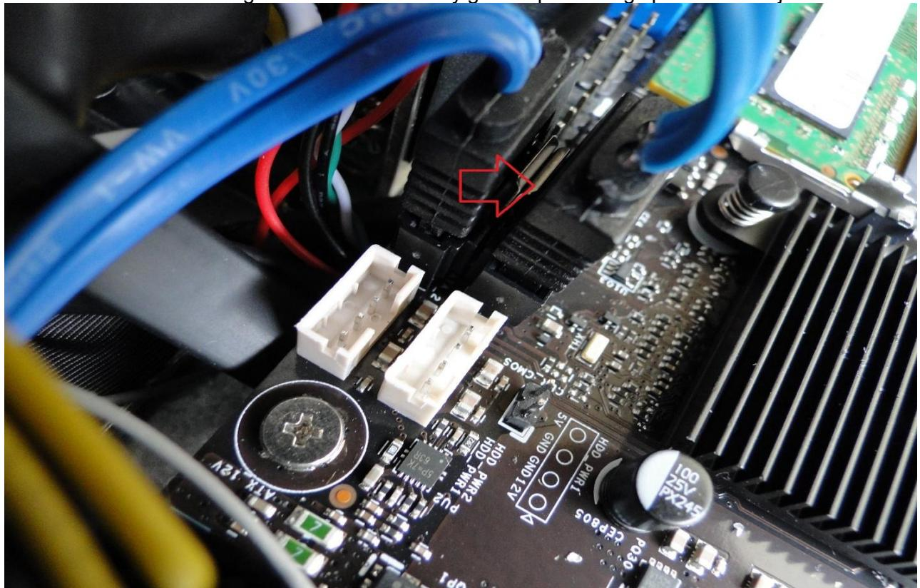
Using a flat screwdriver, press the lock release in the direction indicated by the arrow and pull the cable plug upwards.
