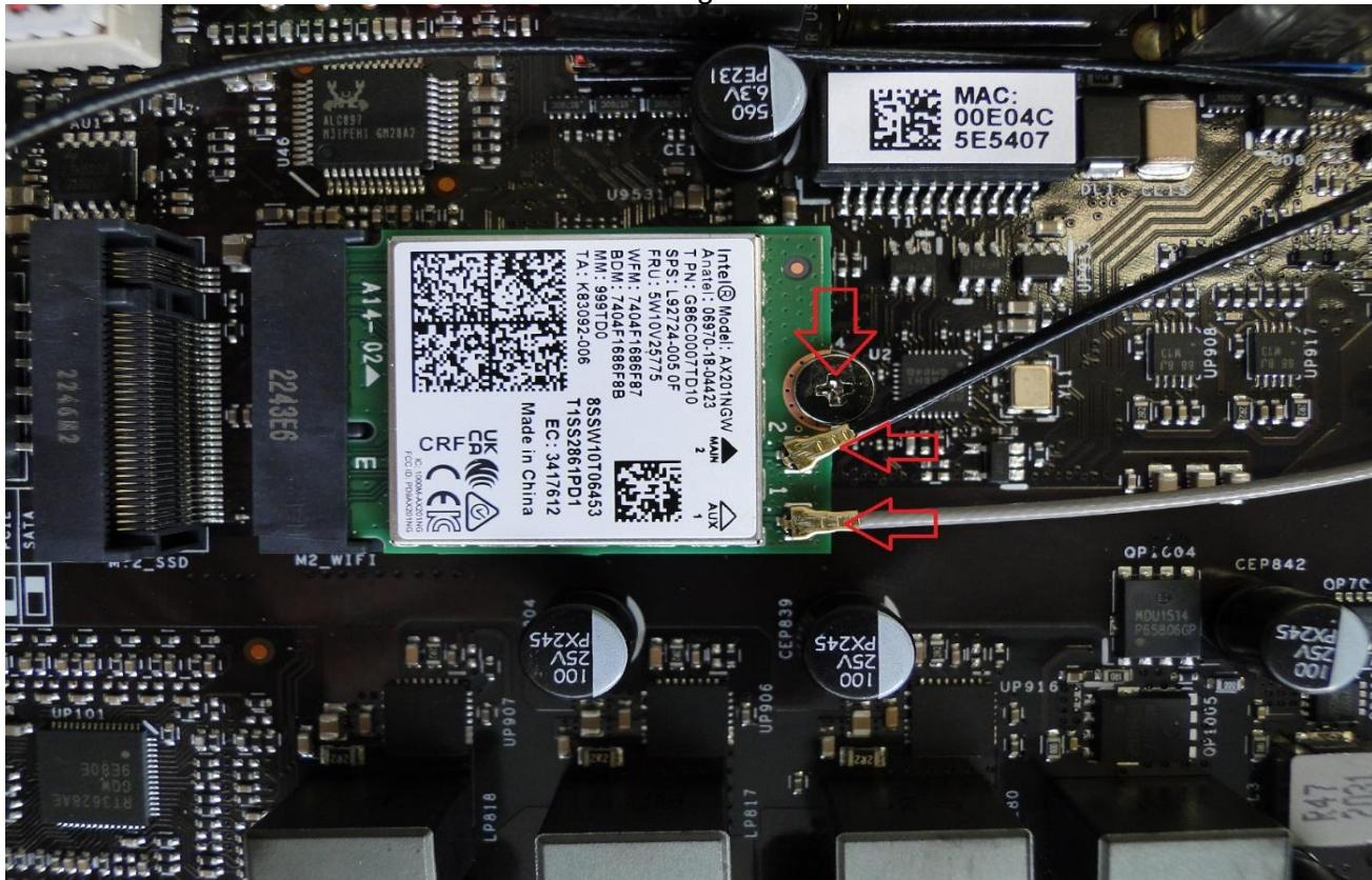
Lift the back of the card up and slide it out of its slot.
