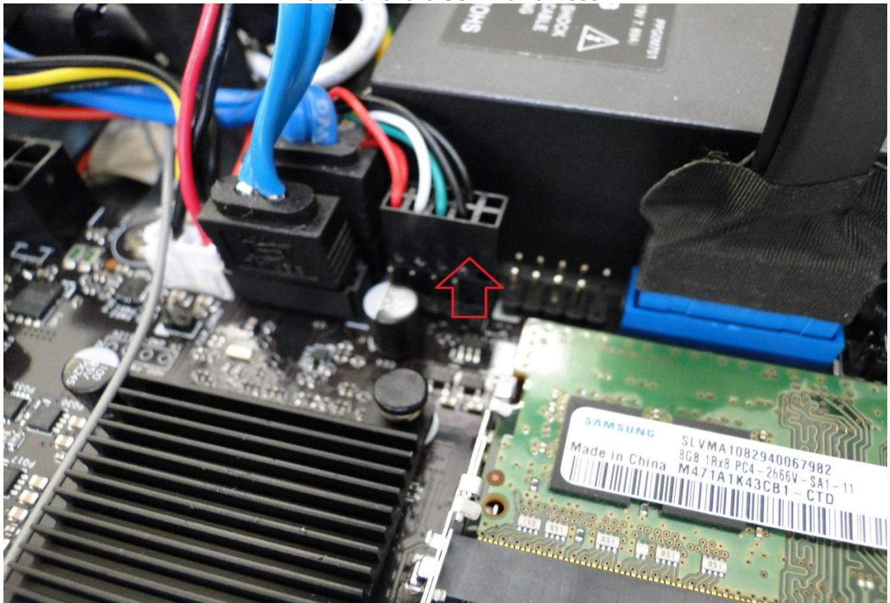
**Removal of the 2.5" SSD power harness and the optical drive**
