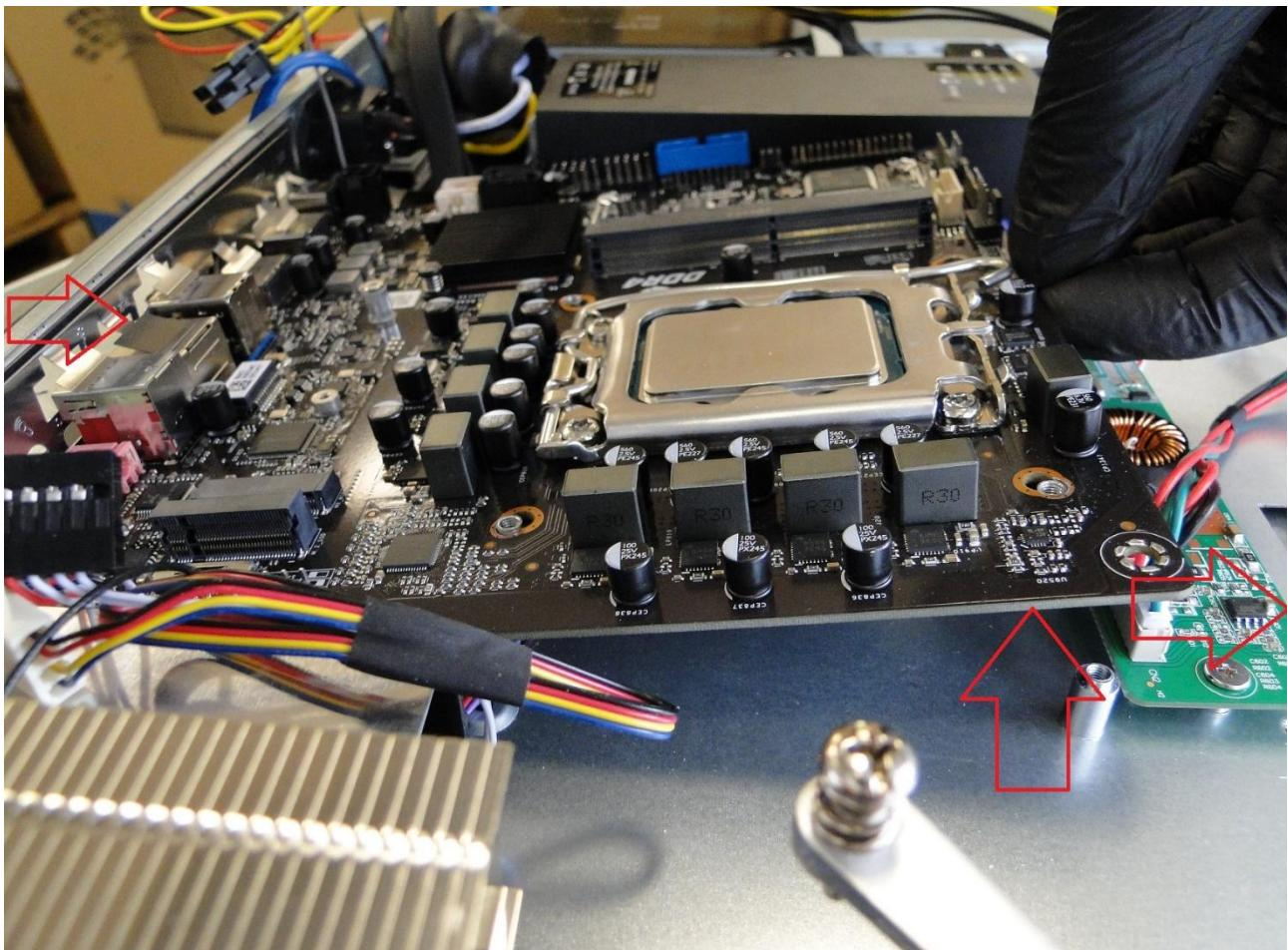
If the new board does not have a processor frame and a BIOS battery, these parts must be disassembled and transferred to the new board. The aforementioned parts are glued down with a double-sided tape.
