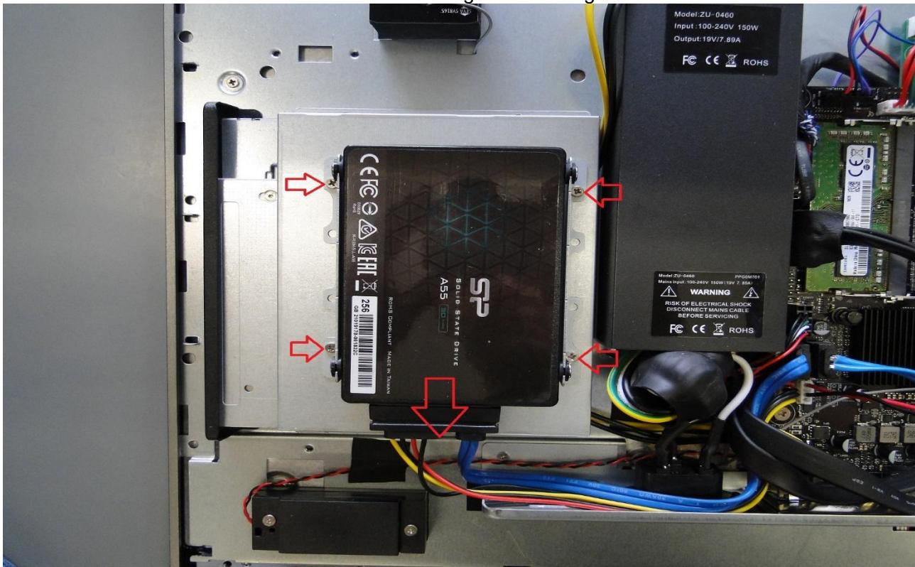
Using a Philips screwdriver, detach the 4 screws securing the 2.5" SSD drive
