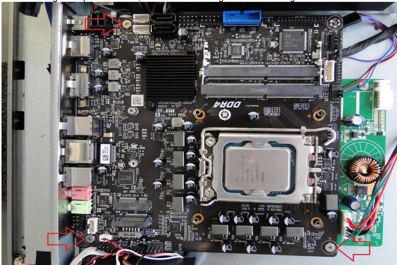
Lift the back of the board up and slide it out of the panel grille.
