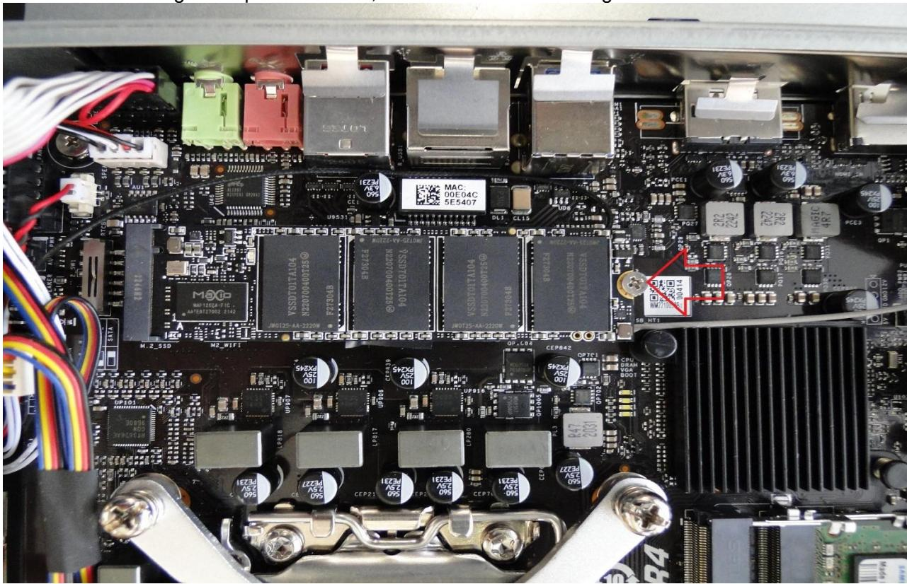
Lift the back of the drive upwards and slide the drive module out of the socket
