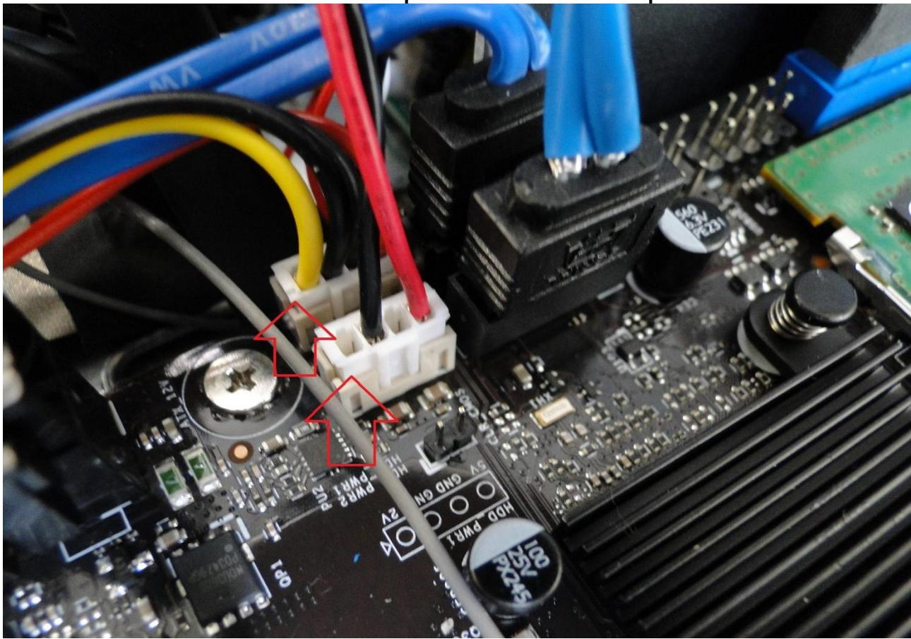
**Removal of the SATA harnesses of the 2.5" SSD disk and the optical drive.**
