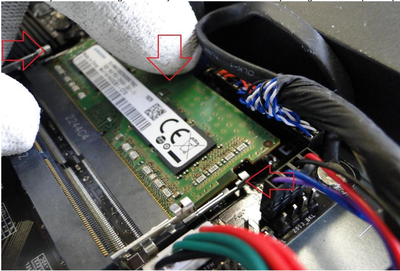
It is possible to carry out an upgrade with an additional module
