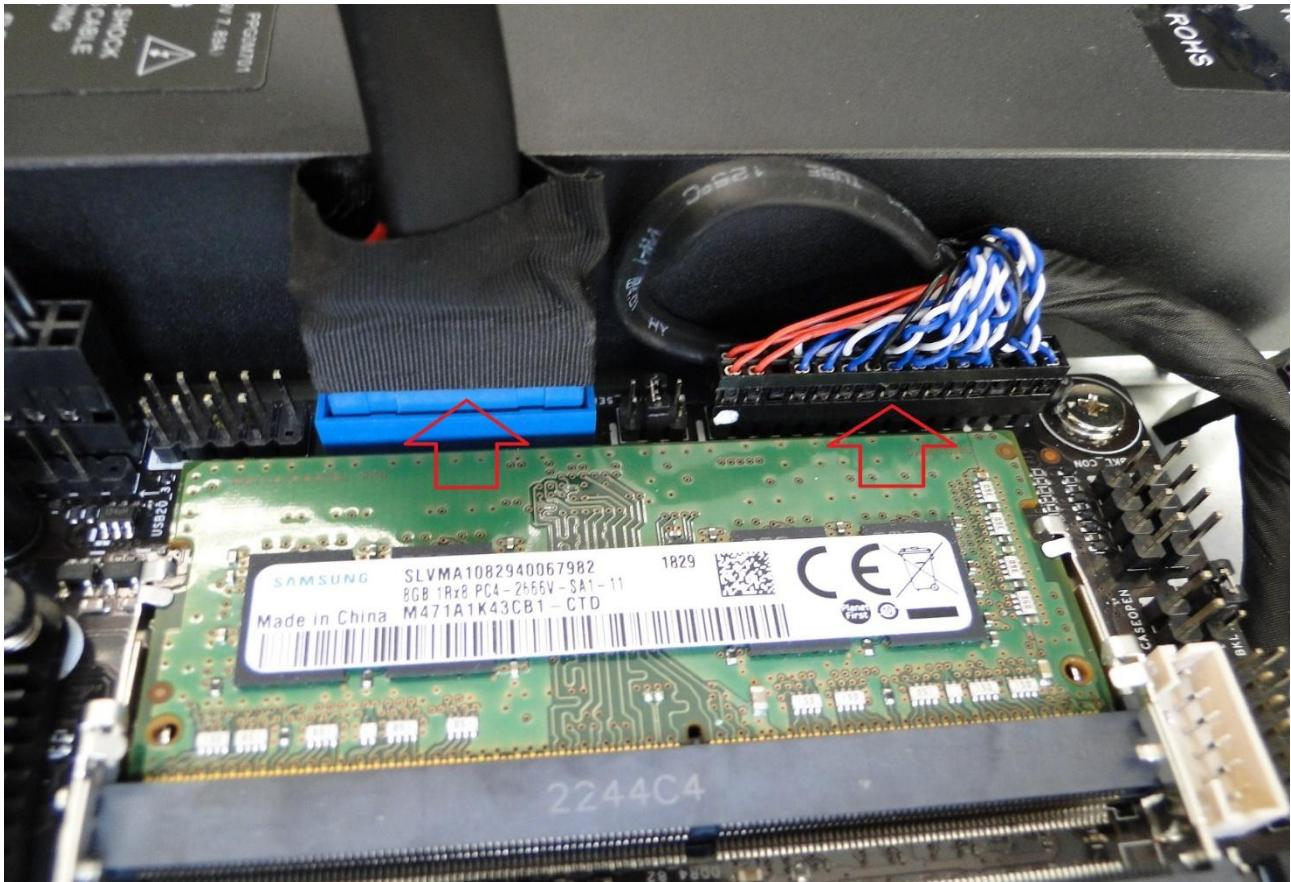
Using a Philips screwdriver, detach the ground wire of the LVDS cable
