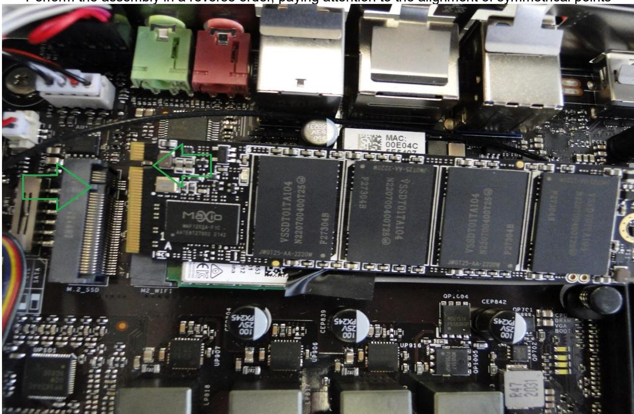
Correct assembly involves inserting the disk into the socket and securing it with a screw
