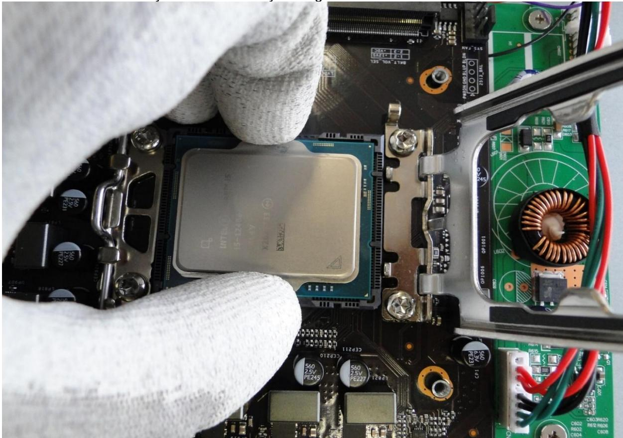
Perform the assembly in a reverse order, paying attention to the alignment of the symmetrical points and the alignment of the CPU and the base
