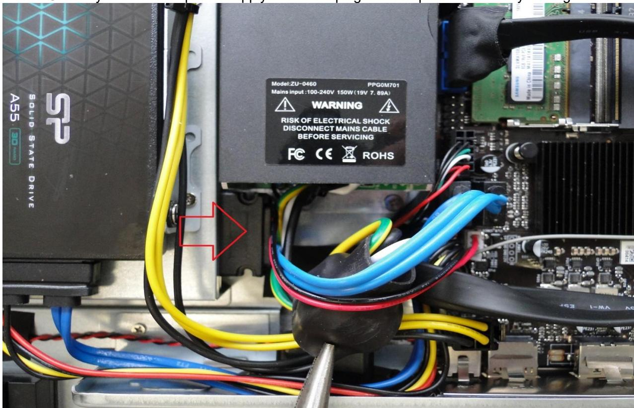
Using a Philips screwdriver, detach the 4 screws securing the power supply.
