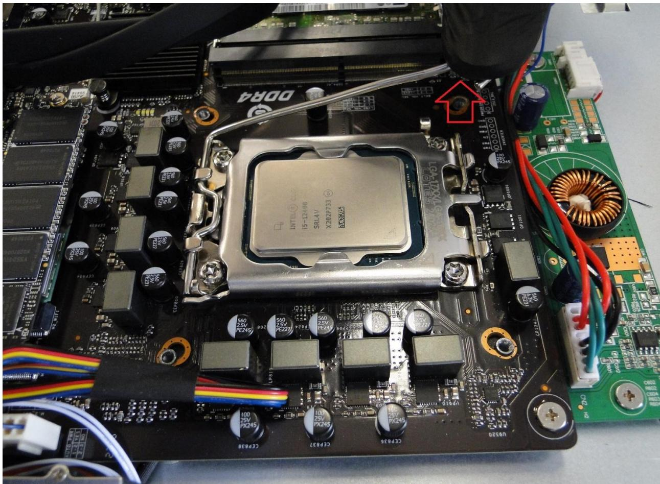
Lift the cover of the CPU socket to a 90 degree angle
