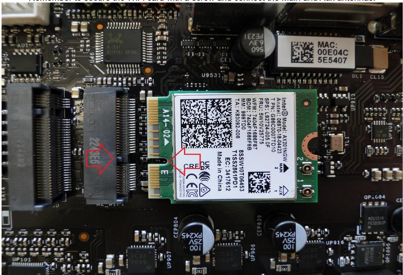
Correct installation involves inserting the card into the slot, securing it with a screw and plugging in the antennas
