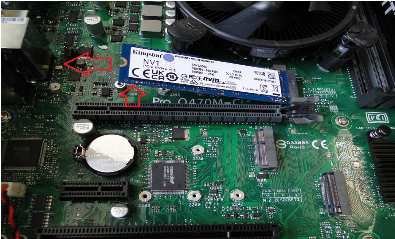
Installation is to be carried out in reverse order, paying attention to the alignment of the drive cutout with the M\_2 slot.
