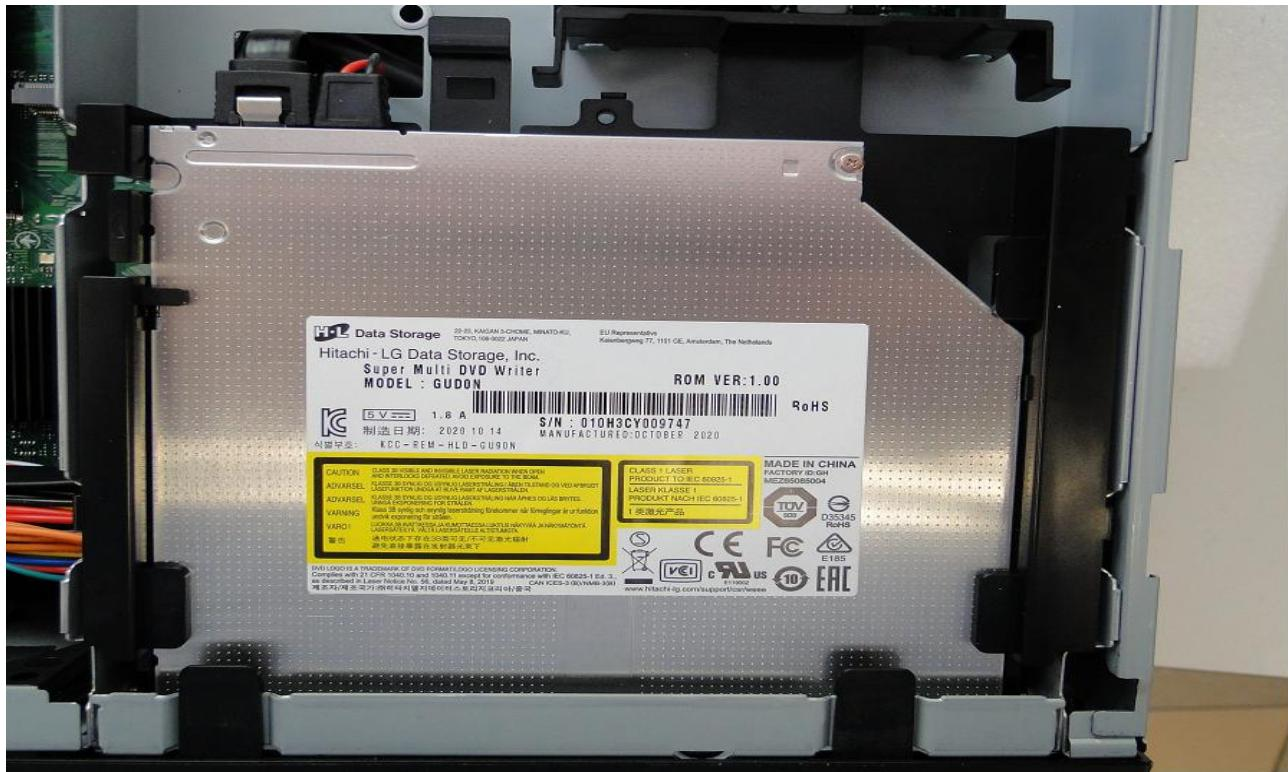
Carefully slide out the power and SATA plugs with your fingers. The SATA cable may have a have a safety feature in the form of a metal ratchet which must be pressed.
