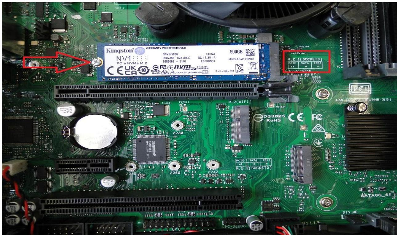
Lift the back of the disk up and slide it out of the slot.
